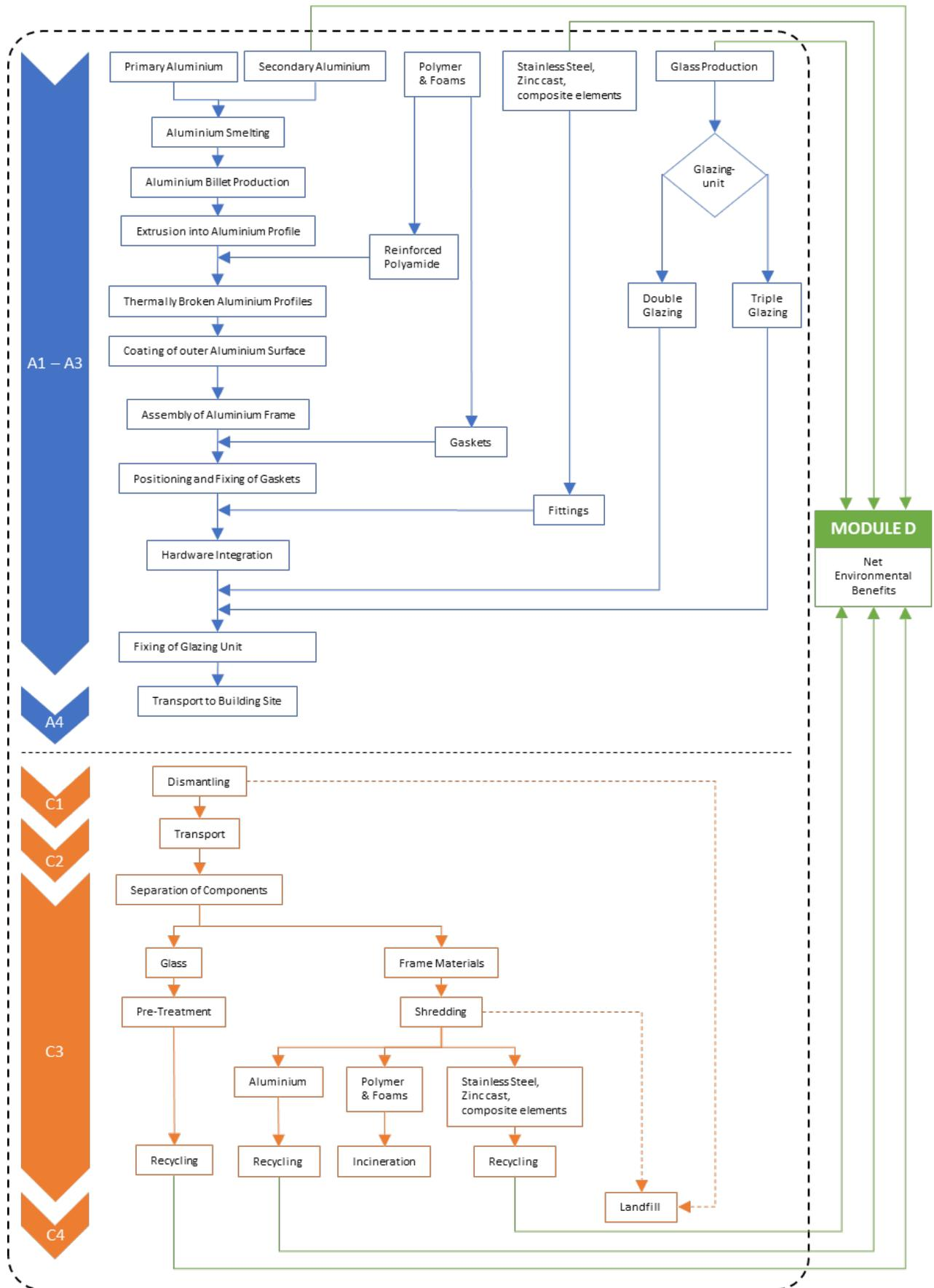
Figure 1 Main production processes and components of the window system
